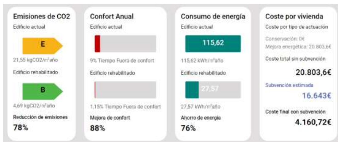
Figure 23.- Scenario 09: Thermal envelope renovation + Photovoltaic
