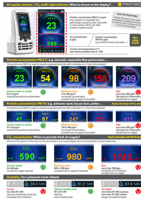
Figure 32. Fact sheet about the indoor environmental quality provided by the Trotec BQ30 monitor.
